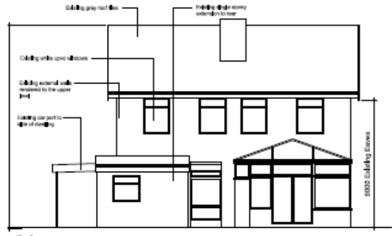
Existing rear elevation
